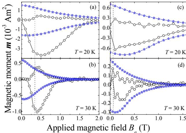
Fig. 1. Magnetization curves of the Fe-sheathed and bare wires for the transverse (a,b) and longitudinal (c,d) field orientations at different temperatures. The curve legend is given in the text.
