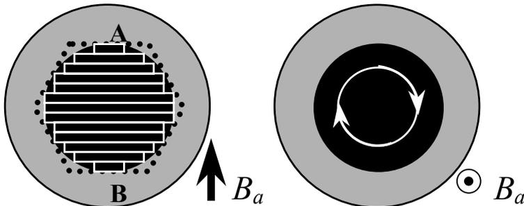
Fig. 2. Electro-magnetic schematics of the sheathed wire cross section in the case of the transverse (left) and longitudinal (right) field orientations. The superconducting core can be approximated as a stack of strips with their own Meissner shielding current confined within each strip. The dotted line shows a hexagonal approximation of the iron sheath. The white circular arrows denote shielding currents.
