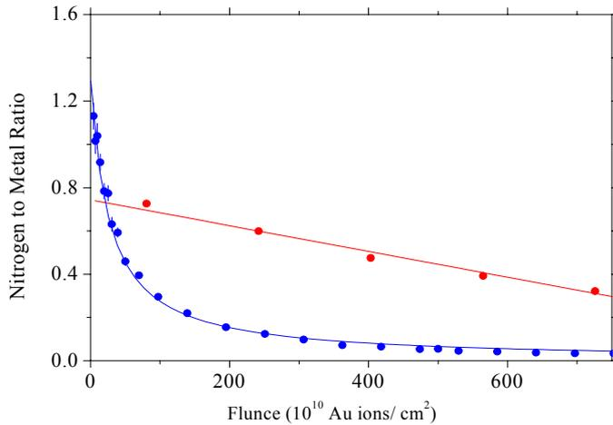
Fig.3: N/Ga (red symbols) and N/In (blue symbols) ratios versus the fluence of projectile ions during ERD analysis for a GaN and an InN film, respectively. The data for GaN can be approximated with a straight line (red). The strong depletion of N in the case of InN is well reproduced by a two-parameter function derived from a depletion model for nitrogen. The best fit with this function is shown as a blue curve.
