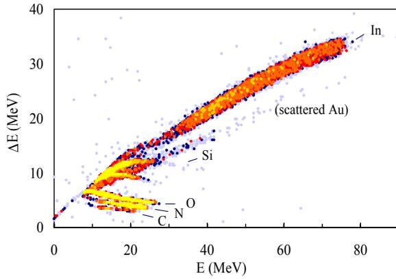
Fig.1: A 2D spectrum from the ERD analysis of a typical polycrystalline InN film grown on glass. The labels indicate groups of events associated with a specific element.
