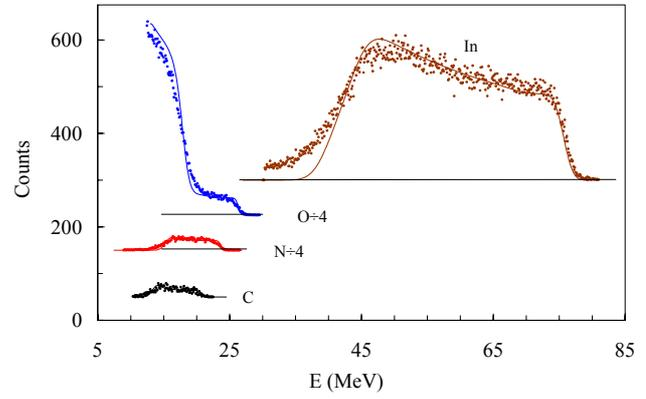
Fig.2: Energy spectra for recoil ions from sample A in comparison with a simulation using the program SIMNRA, which agrees well with the data. For clarity the spectra have been shifted upwards by constant numbers of counts.
