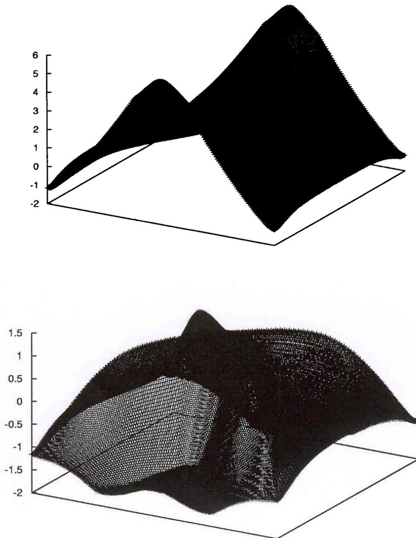
Fig. 6. Energy values in eV close to the Fermi surface (plane through z axis at 0 eV) in the plane containing the lines  $\Sigma$  and lines  $\Lambda$  (compare Fig. 2) for two different energy bands that both cross the Fermi surface.
