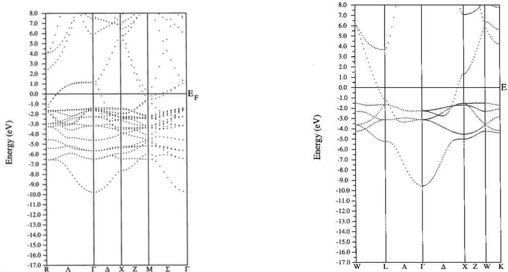
Fig. 3 Comparison of electronic band structure for  $\text{Cu}_3\text{Au}$  (left) with Cu (right). Note that in the case of  $\text{Cu}_3\text{Au}$  more than one band intersects the Fermi level denoted by  $E_F$ . The principal symmetry directions are as denoted in Figs. 1 and 2 respectively.
