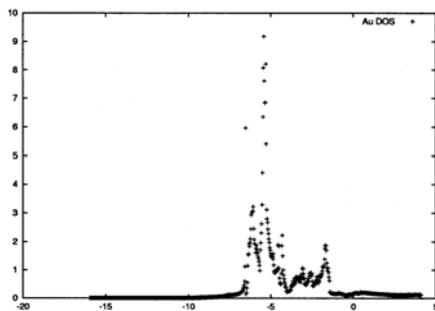
Fig. 4. Contribution of Cu and Au sites in  $\text{Cu}_3\text{Au}$  total DOS versus energy in eV.
