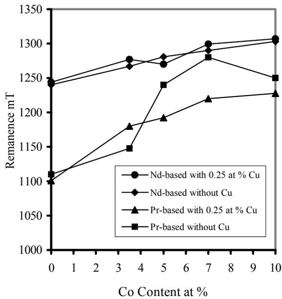
Fig. 3 Effect of cobalt content on the remanence of magnets containing 0.25 at % Cu
