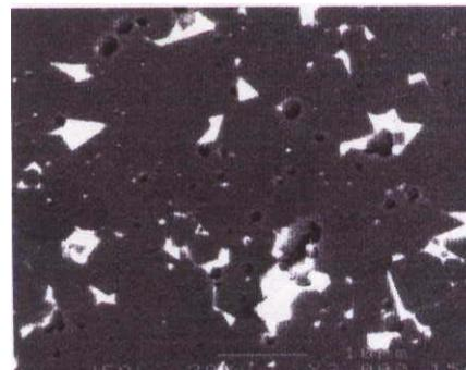
Fig. 2 Back scattered electron image of Pr-based magnet blended with 5 at % Co-0.25 at % Cu. Labels indicate (a)  $\text{Pr}_2\text{Fe}_{14}\text{B}$ , (b)  $\text{Pr}_6\text{Fe}_{13}\text{Cu}$  (c)  $\text{PrFe}_4\text{B}_4$ , (d)  $\text{Pr}_3(\text{Co,Fe})$
