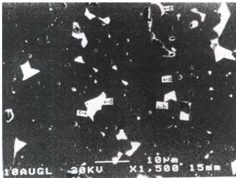
Fig. 1 Back scattered electron image of Nd-based magnet blended with 5 at % Co - 0.25 at % Cu. Labels indicate (a)  $\text{Nd}_2\text{Fe}_{14}\text{B}$ , (b)  $\text{NdFe}_4\text{B}_4$ , (c) Nd-rich, (d)  $\text{Nd}_3\text{CoFe}$ , and (e) Cu-rich
