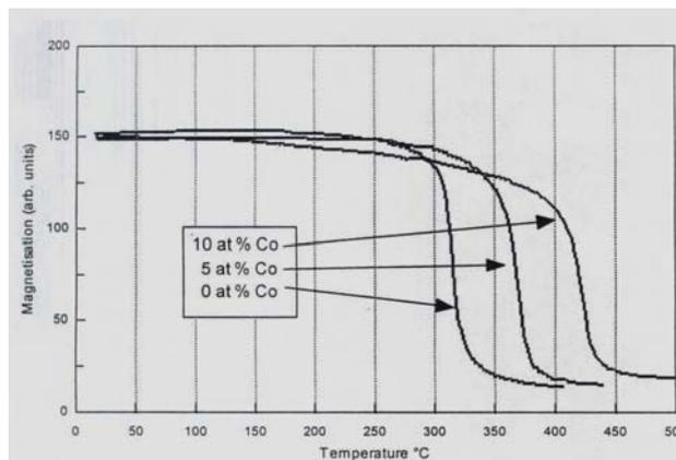
Fig. 5 Effect of cobalt content on the Curie temperature of Nd-based magnets with 0.25 at % copper
