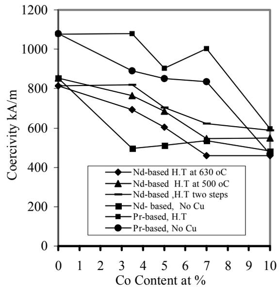
Fig.4 Effect of cobalt content and heat treatment temperature on the coercivity of magnets containing 0.25 at % Cu
