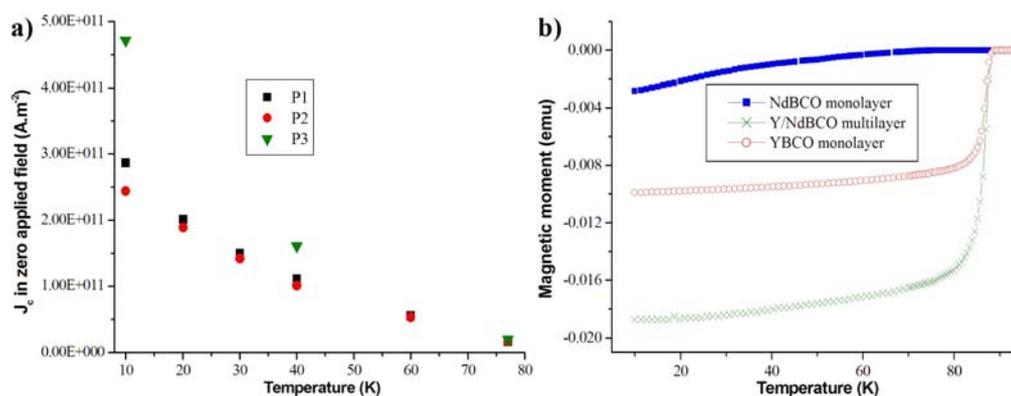
Figure 3. a) Magnetic  $J_c$  as a function of the temperature for the three samples produced by PLD, b) Magnetic moment as a function of the temperature for P3 and NdBCO and YBCO monolayer films deposited in the same conditions.
