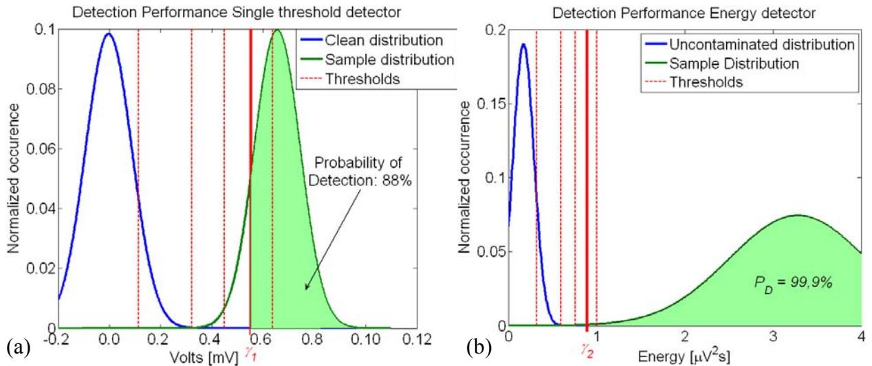
Figure 2. Probability density functions of (a) Single threshold detector (b) Energy detector. The vertical red lines mark the thresholds for  $P_{FA}$  from  $10^{-1}$  to  $10^{-12}$  from left to right.
