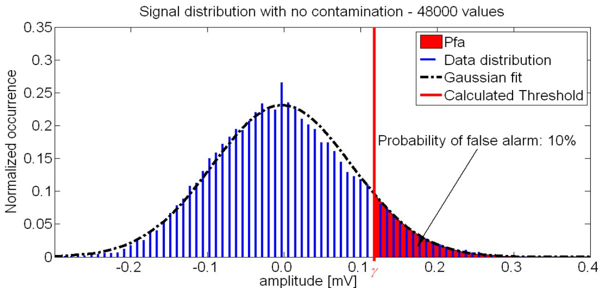
Figure 1. Data distribution over 240 sec without contamination; threshold calculated for  $P_{FA} = 10\%$ .
