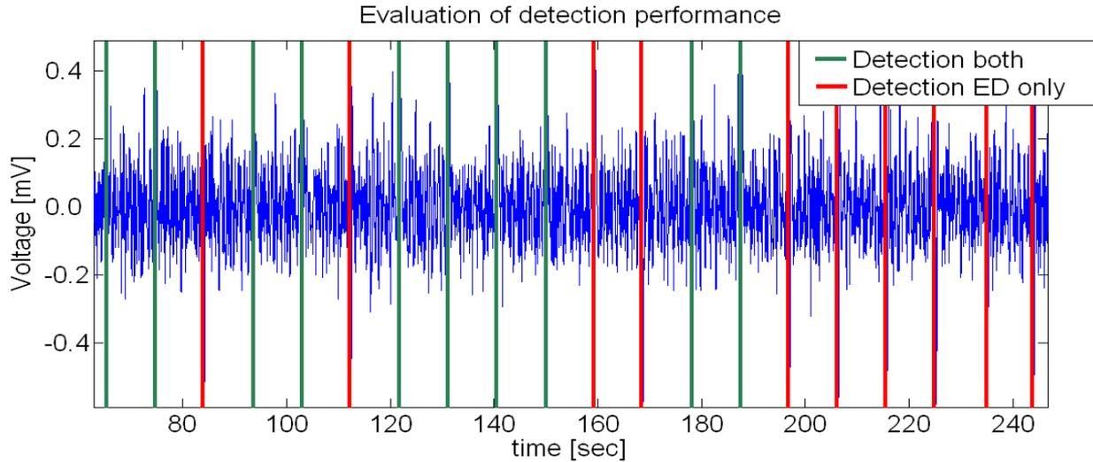
Figure 3. For  $P_{FA} = 10^{-12}$  ED detected all 20 passes of the sample whereas the STD (green lines) detected the sample only 50% of the time.
