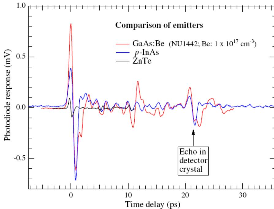
**Figure 4.** A comparison between the three emitter classes.
