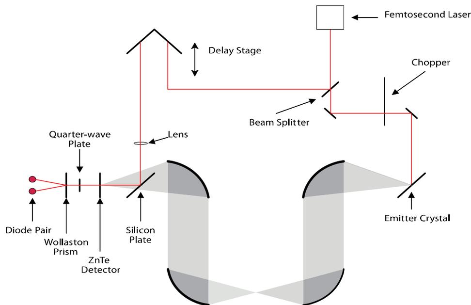
**Figure 1.** Diagram of the time-domain spectroscopy apparatus.
