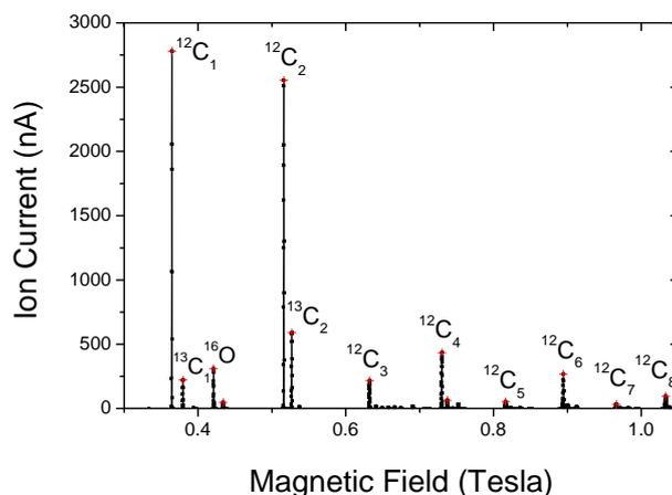
Fig. 4. A typical mass spectrum of carbon monomer and clusters from SNICS ion source. (The small peaks in the mass spectra are likely the clusters including  $^{13}\text{C}$ ).
