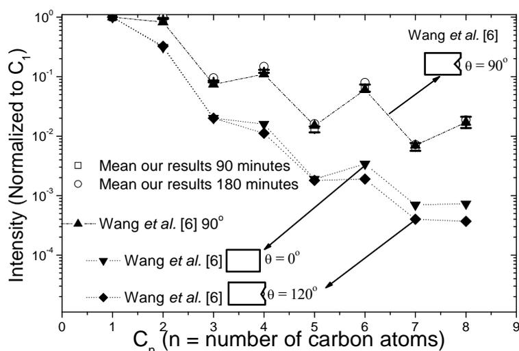
Fig. 5. Comparison of our data of all graphite cathodes with the Wang *et al.* data [6].
