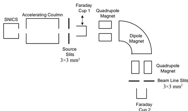
Fig. 2 Schematic diagrams of 150 KeV ion implanter and SNICS ion source.
