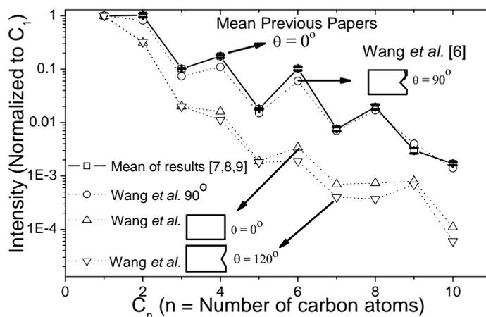
Fig. 1. Mean value of measured carbon cluster currents for solid graphite cathodes [7, 8, 9] compared with results by Wang *et al.* [6] results for three different cathode geometries including conical recess with opening angle of  $\theta = 90^\circ$  and  $\theta = 120^\circ$ .
