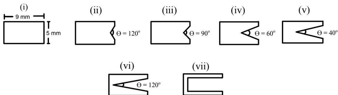
Fig. 3. Cross sectional drawings of the different graphite cathodes geometries studied in this work.
