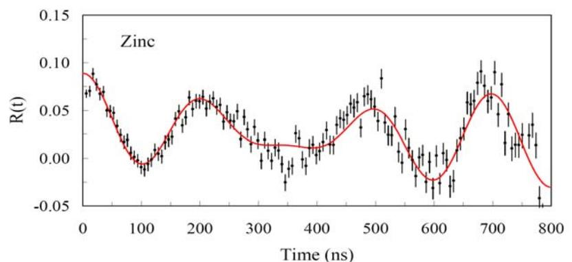
Fig. 1. Measured ratio function  $R(t)$  for  $^{100}\text{Rh}$  in zinc. The fitted curve is shown in red.
