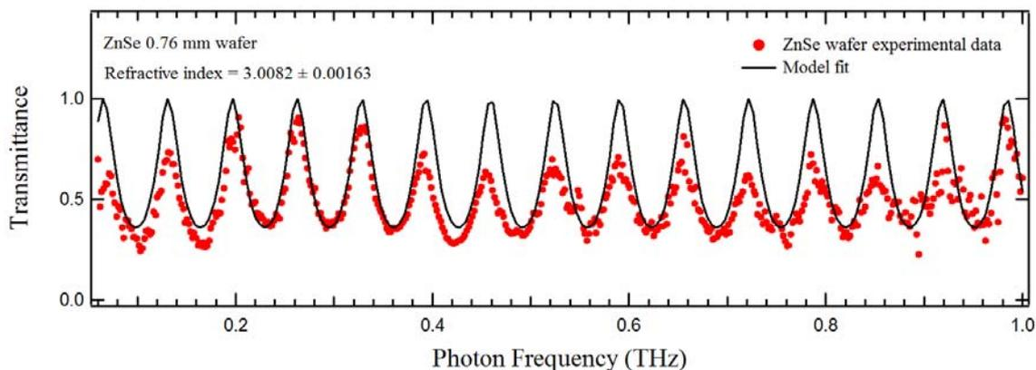
Fig. 4. Experimental transmittance of ZnSe sample fitted with Drude model for determining refractive index.
